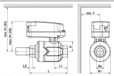
H1/X1: without spindle extension CQ H2/X2: with spindle extension CQ (ZCQ-E)
